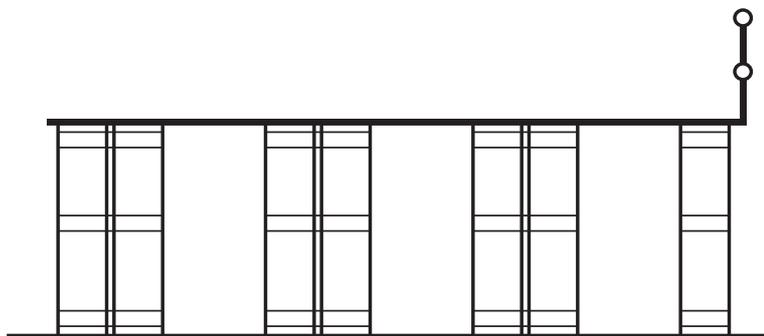
Figure 3 — Over-rack mezzanine floor
