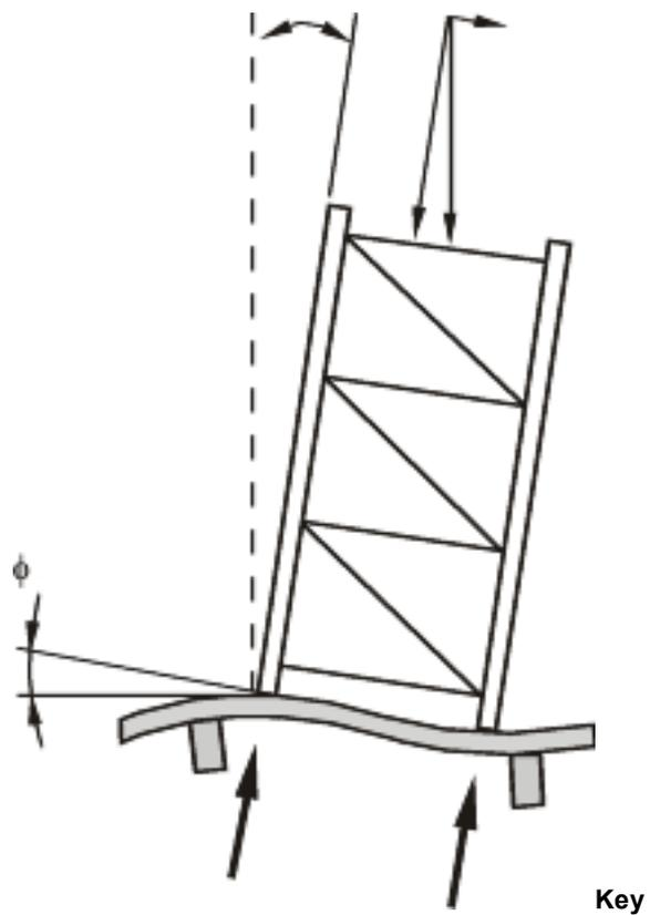
$\phi$  floor slope under the rack frame
