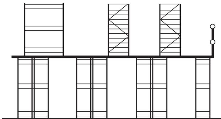
Figure 4 — Over-rack mezzanine floor supporting shelving
