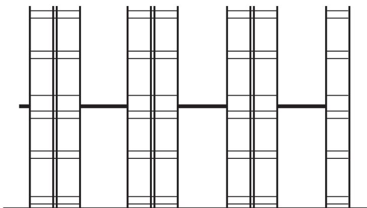
Figure 6 — Walkways suspended between the upright frames
